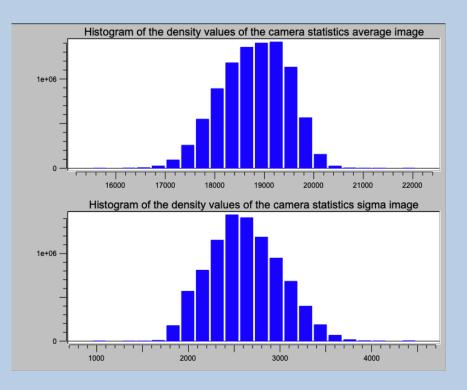
The histograms usually have a Gaussian like shape. In case of detector errors (blind or dark pixels, for example) these can easily be seen as vertical lines.
