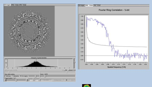
In contrast to the FRC/FSC curve the FRI/FSI plots also show the estimated resolution value in case FRI/FSI curve and the ½-bit threshold curve intersect:
