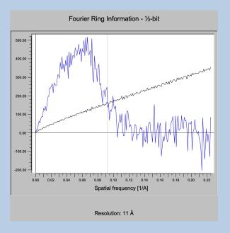
The ½-bit information curve indicates where a sufficient amount of data is collected to allow a direct interpretation at that resolution level. The overall resolution achieved is estimated by the intersection of the FRI/FSI curve (blue) and the 1/2 Bit curve (black).
